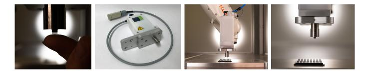
Through a combination of vacuum and ultrasound, attractive and repulsive forces act simultaneously on the workpiece and keep it at a distance, even when gripping from above. As a result, no contamination or micro-scratches can occur on the small part.
