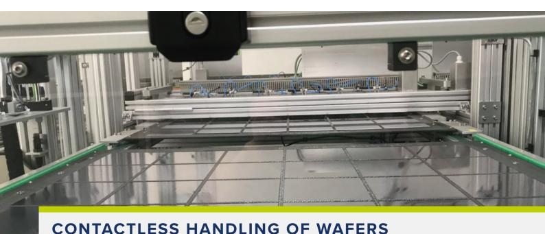
The modular Waferhandling-System facilitates all possible handling processes of wafers. Loading and unloading, conveying, gripping, inspecting, sorting
